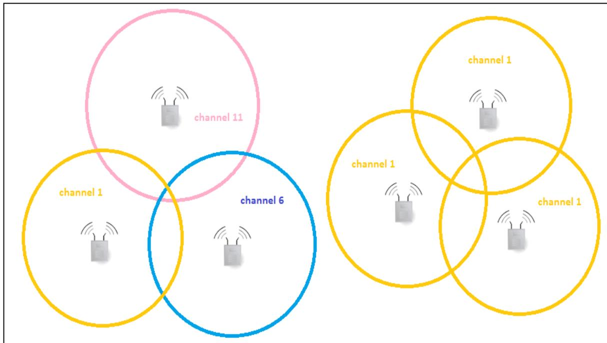
Let's have a look at the theoretical design of the 802.11b network with 3 cells, adjacent to each other as shown in the above picture. Design on the left is composed of 3 non-overlapping channels - it means that frames sent by APs and its clients in particular cell, will not interfere with communication in other cells. On the right, we have a completely opposite situation, all the frames flying around on the same channel leads to collisions and degrade the wireless performance significantly.
