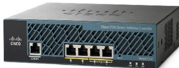
This is the situation, where the concept of wireless controller comes into play. It is the "Mastermind" behind all the wireless network operation. This centralized server which has the IP connectivity to all the AP's on the network making it easy to manage all of them globally from the single management platform, push configuration templates, monitor users from all the AP's in real time and so on.
