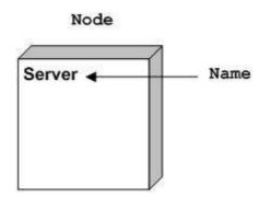
Node is used to represent physical part of a system like server, network etc.
