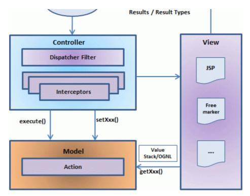
The above diagram depicts the  $\underline{\mathbf{M}}$  odel,  $\underline{\mathbf{V}}$  iew and  $\underline{\mathbf{C}}$  ontroller to the Struts2 high level architecture. The controller is implemented with a Struts2 dispatch servlet filter as well as interceptors, the model is implemented with actions, and the view as a combination of result types and results. The value stack and OGNL provide common thread, linking and enabling integration between the other components.
