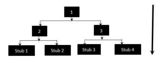
The above diagrams clearly states that Modules 1, 2 and 3 are available for integration, whereas, below modules are still under development that cannot be integrated at this point of time. Hence, Stubs are used to test the modules. The order of Integration will be:
