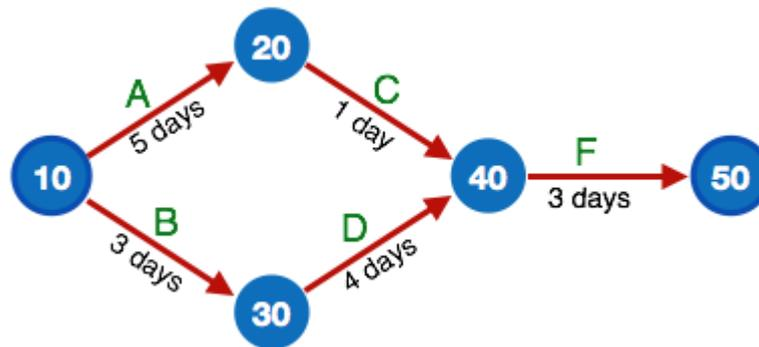
Events are shown as numbered nodes. They are connected by labeled arrows depicting the sequence of tasks in the project.
