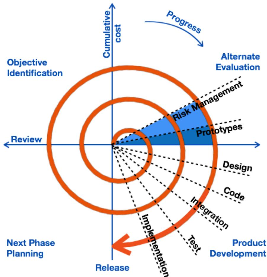
This model considers risk, which often goes un-noticed by most other models. The model starts with determining objectives and constraints of the software at the start of one iteration. Next phase is of prototyping the software. This includes risk analysis. Then one standard SDLC model is used to build the software. In the fourth phase of the plan of next iteration is prepared.
