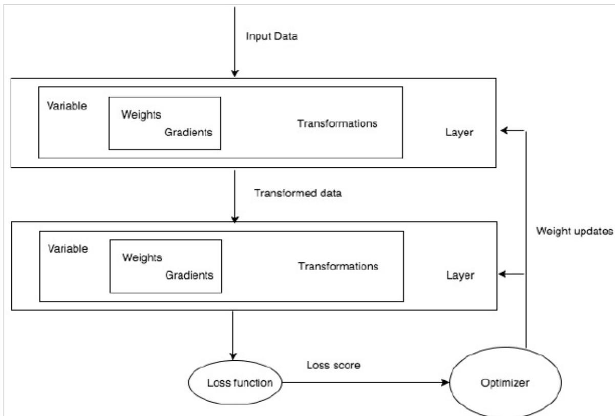
With respect to the above diagram, any deep learning algorithm involves getting the input data, building the respective architecture which includes a bunch of layers embedded in them.
