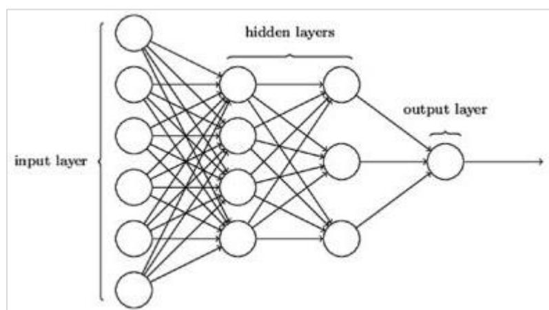
The layers between input and output are referred to as hidden layers, and the density and type of connections between layers is the configuration. For example, a fully connected configuration has all the neurons of layer  $L$  connected to those of  $L+1$ . For a more pronounced localization, we can connect only a local neighbourhood, say nine neurons, to the next layer. Figure 1-9 illustrates two hidden layers with dense connections.
