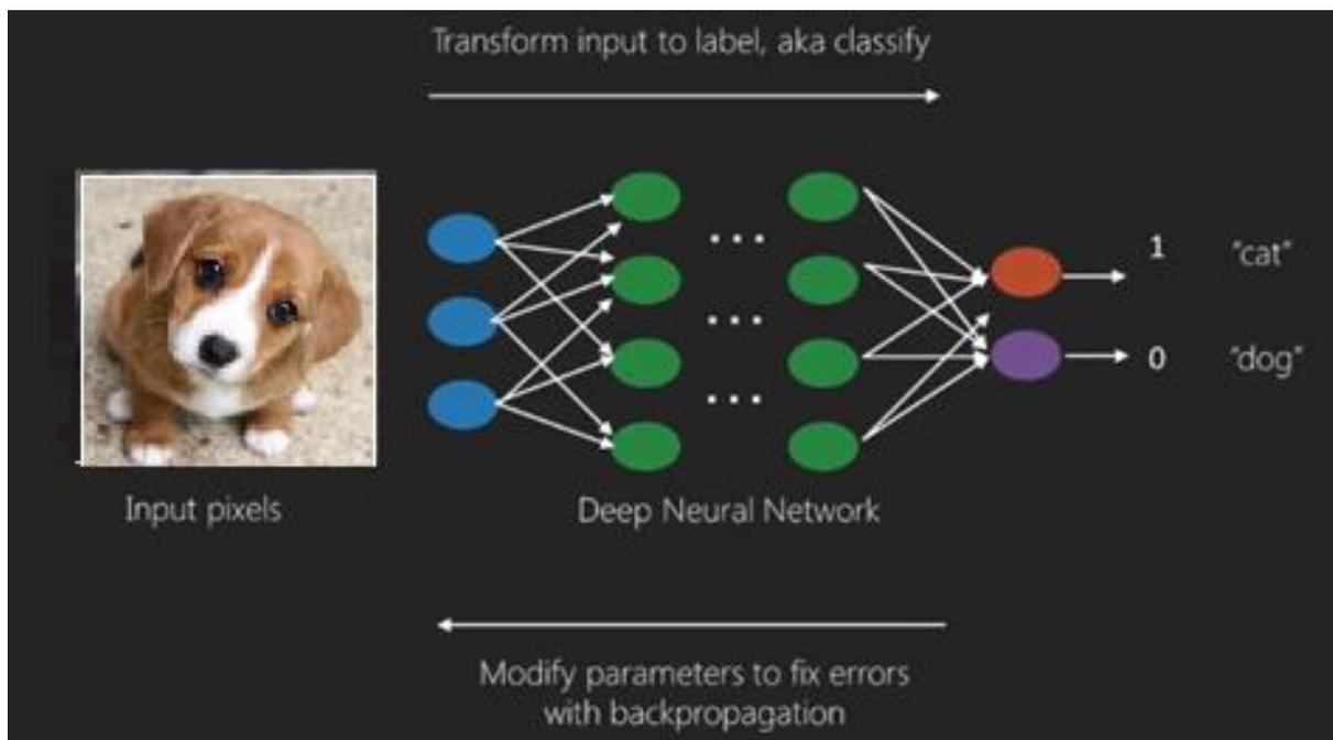
Here we apply backpropagation algorithm to get correct output prediction.
