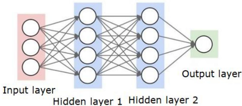
The circles are neurons or nodes, with their functions on the data and the lines/edges connecting them are the weights/information being passed along.
