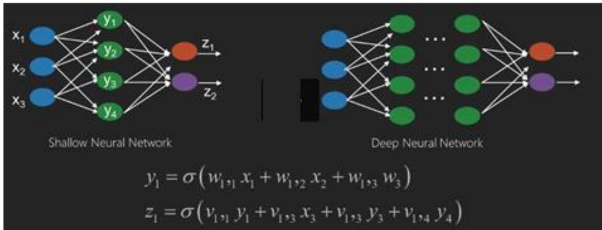
Neural networks are functions that have inputs like  $x_1, x_2, x_3$ ...that are transformed to outputs like  $z_1, z_2, z_3$  and so on in two (shallow networks) or several intermediate operations also called layers (deep networks).
