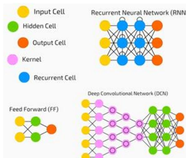
Neural networks are widely used in supervised learning and reinforcement learning problems. These networks are based on a set of layers connected to each other.
