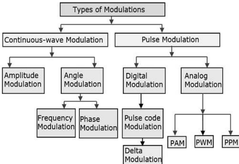
The types of modulations are broadly classified into continuous-wave modulation and pulse modulation.
