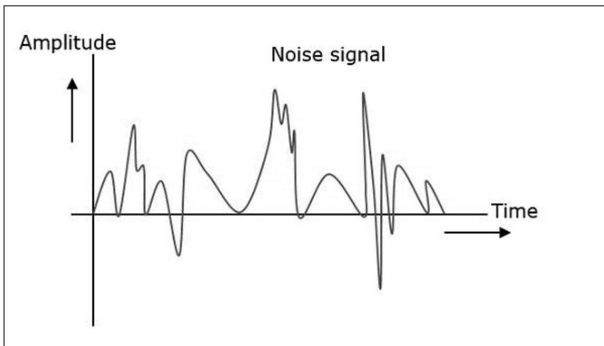
Hence, it is understood that noise is some signal which has no pattern and no constant frequency or amplitude. It is quite random and unpredictable. Measures are usually taken to reduce it, though it can't be completely eliminated.
