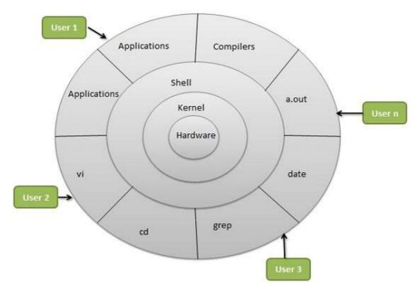
Linux System Architecture is consists of following layers
