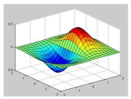
You can also use the **mesh** command to generate a three-dimensional surface. However, the **surf** command displays both the connecting lines and the faces of the surface in color, whereas, the **mosh** command croates a wireframe surface with colored lines connecting the defining points. Loading [MathJax]/jax/output/HTML-CSS/jax.js
