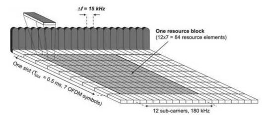
Each user is allocated a number of so-called resource blocks in the time.frequency grid. The more resource blocks a user gets, and the higher the modulation used in the resource elements, the higher the bit-rate. Which resource blocks and how many the user gets at a given point in time depend on advanced scheduling mechanisms in the frequency and time dimensions.
