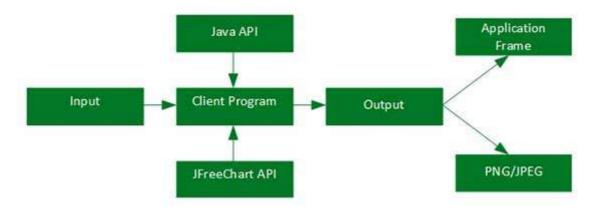
The client program receives user data and then it make use standard Java and JFreeChart APIs based on requirements to generate the output in the form of either a frame, which can be displayed directly inside the application or independently in the image formats such as JPEG or PNG.
