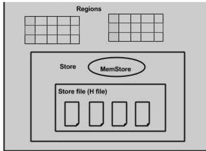
The store contains memory store and HFiles. Memstore is just like a cache memory. Anything that is entered into the HBase is stored here initially. Later, the data is transferred and saved in Hfiles as blocks and the memstore is flushed.
