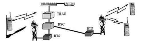
The MS and the BSS communicate across the Um interface. It is also known as the *air interface* or the *radio link*. The BSS communicates with the Network Service Switching *NSS* center across the *A* interface.
