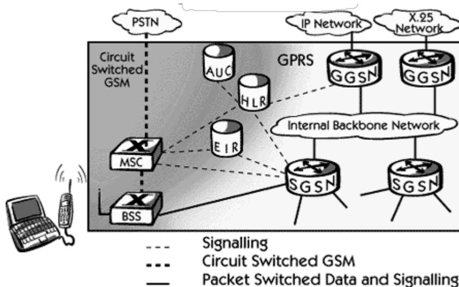
GPRS attempts to reuse the existing GSM network elements as much as possible, but to effectively build a packet-based mobile cellular network, some new network elements, interfaces, and protocols for handling packet traffic are required.
