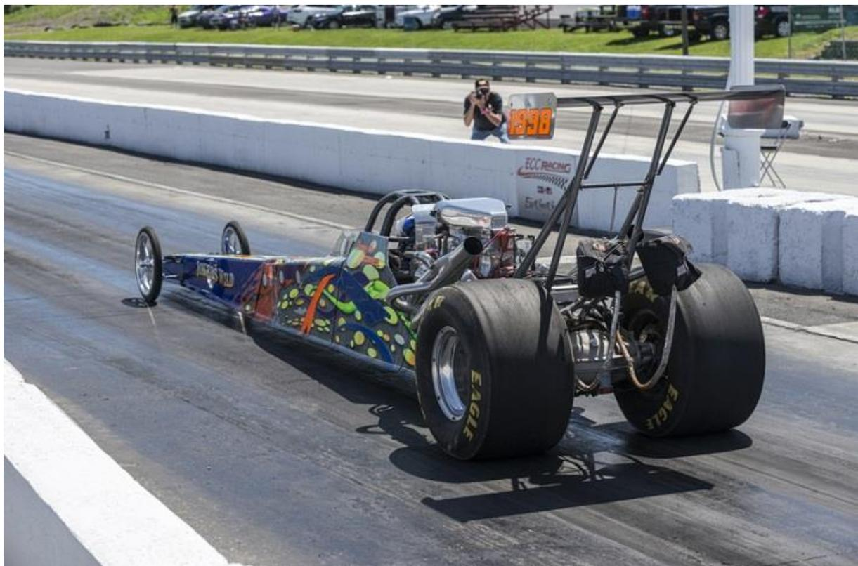
A supercharged methanol-burning engine might be used. A combination of an injected nitro methane can also be used as a fuel. These cars can pick up the speed of 280 mph in 5.1s.
