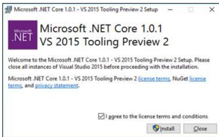
**Step 8:** Check the checkbox and click Install.
