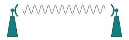
Microwave antennas concentrate the waves making a beam of it. As shown in picture above, multiple antennas can be aligned to reach farther. Microwaves have higher frequencies and do not penetrate wall like obstacles.
