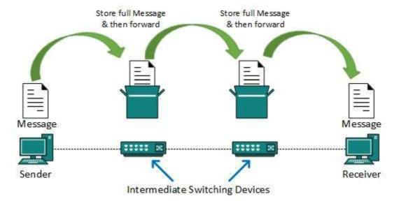
This technique was considered substitute to circuit switching. As in circuit switching the whole path is blocked for two entities only. Message switching is replaced by packet switching. Message switching has the following drawbacks:
