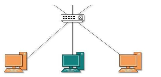
In this diagram, different VLANs are depicted in different color codes. Hosts in one VLAN, even if connected on the same Switch cannot see or speak to other hosts in different VLANs. VLAN is Layer-2 technology which works closely on Ethernet. To route packets between two different Loading [MathJax]/jax/output/HTML-CSS/jax.js
