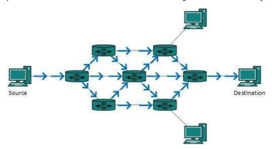
This method is easy on router's CPU but may cause the problem of duplicate packets received from peer routers.
