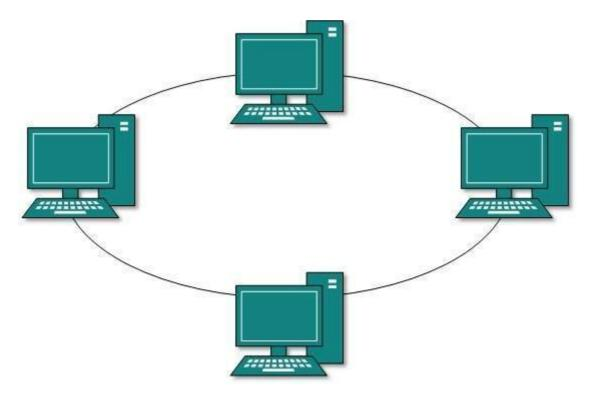
Failure of any host results in failure of the whole ring. Thus, every connection in the ring is a point of failure. There are methods which employ one more backup ring.
