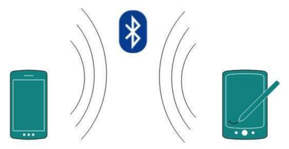
For example, Piconet is Bluetooth-enabled Personal Area Network which may contain up to 8 devices connected together in a master-slave fashion.
