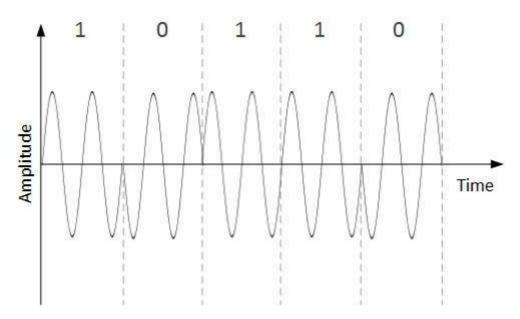
When a new binary symbol is encountered, the phase of the signal is altered. Amplitude and frequency of the original carrier signal is kept intact.
