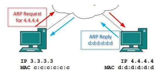
To know the MAC address of remote host on a broadcast domain, a computer wishing to initiate communication sends out an ARP broadcast message asking, "Who has this IP address?" Because it is a broadcast, all hosts on the network segment *broadcastdomain* receive this packet and process it. ARP packet contains the IP address of destination host, the sending host wishes to talk to. When a host receives an ARP packet destined to it, it replies back with its own MAC address.
