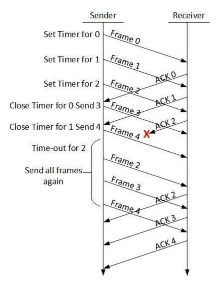
The sending-window size enables the sender to send multiple frames without receiving the acknowledgement of the previous ones. The receiving-window enables the receiver to receive multiple frames and acknowledge them. The receiver keeps track of incoming frame's sequence number.
