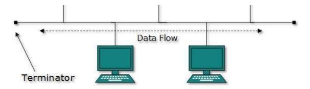
Both ends of the shared channel have line terminator. The data is sent in only one direction and as soon as it reaches the extreme end, the terminator removes the data from the line.
