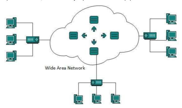
WAN may use advanced technologies such as Asynchronous Transfer Mode *ATM*, Frame Relay, and Synchronous Optical Network *SONET*. WAN may be managed by multiple administration.
