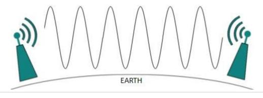
Radio waves of high frequencies are prone to be absorbed by rain and other obstacles. They use lonosphere of earth atmosphere. High frequency radio waves such as HF and VHF bands are spread upwards. When they reach lonosphere, they are refracted back to the earth.
