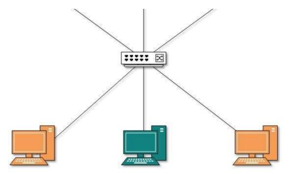
In this diagram, different VLANs are depicted in different color codes. Hosts in one VLAN, even if connected on the same Switch cannot see or speak to other hosts in different VLANs. VLAN is Layer-2 technology which works closely on Ethernet. To route packets between two different VLANs a Layer-3 device such as Router is required.
