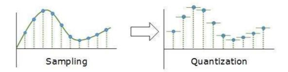
Sampling yields discrete form of continuous analog signal. Every discrete pattern shows the amplitude of the analog signal at that instance. The quantization is done between the maximum amplitude value and the minimum amplitude value. Quantization is approximation of the instantaneous analog value.
