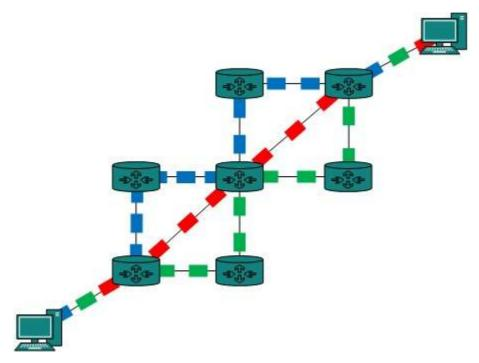
Packet switching enhances line efficiency as packets from multiple applications can be multiplexed over the carrier. The internet uses packet switching technique. Packet switching
