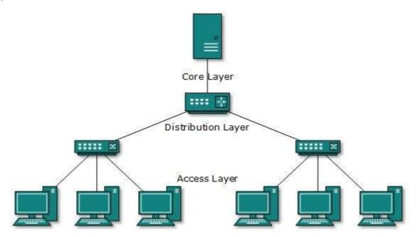
All neighboring hosts have point-to-point connection between them. Similar to the Bus topology, if the root goes down, then the entire network suffers even. though it is not the single point of failure. Every connection serves as point of failure, failing of which divides the network into unreachable segment.
