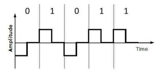
RZ uses three voltage levels, positive voltage to represent 1, negative voltage to represent 0 and zero voltage for none. Signals change during bits not between bits.
