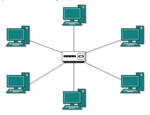
As in Bus topology, hub acts as single point of failure. If hub fails, connectivity of all hosts to all other hosts fails. Every communication between hosts, takes place through only the hub.Star topology is not expensive as to connect one more host, only one cable is required and configuration is simple.
