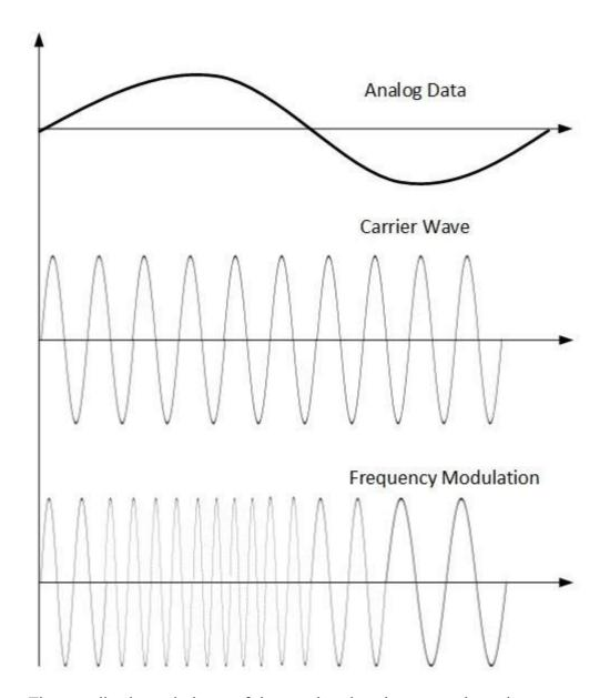
The amplitude and phase of the carrier signal are not altered.
