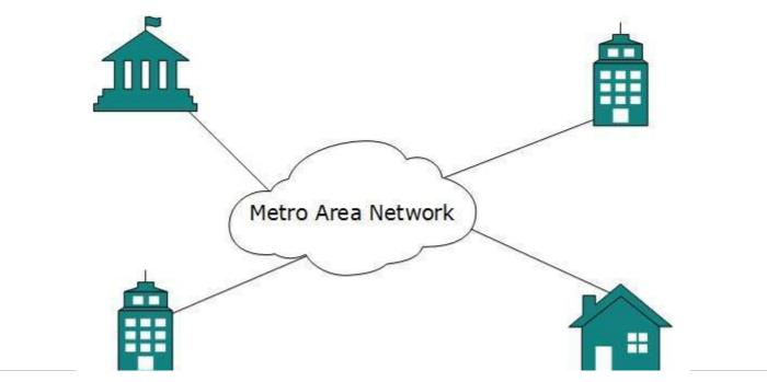
Backbone of MAN is high-capacity and high-speed fiber optics. MAN works in between Local Area Network and Wide Area Network. MAN provides uplink for LANs to WANs or internet.
