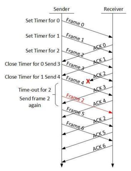
In Selective-Repeat ARQ, the receiver while keeping track of sequence numbers, buffers the frames in memory and sends NACK for only frame which is missing or damaged.
