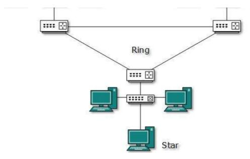
The above picture represents an arbitrarily hybrid topology. The combining topologies may contain attributes of Star, Ring, Bus, and Daisy-chain topologies. Most WANs are connected by means of Dual-Ring topology and networks connected to them are mostly Star topology networks. Internet is the best example of largest Hybrid topology
