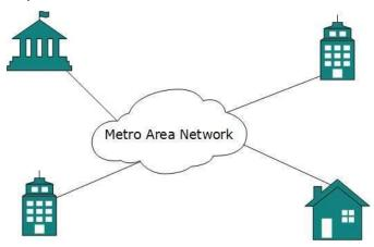
Backbone of MAN is high-capacity and high-speed fiber optics. MAN works in between Local Area Network and Wide Area Network. MAN provides uplink for LANs to WANs or internet.
