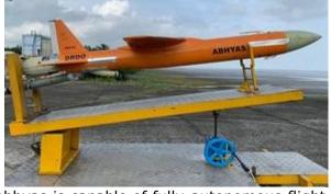
also be used as a decoy aircraft, if needed. Abhyas is capable of fully-autonomous flight and runs on a gas turbine engine.
