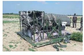
Main canopies, five Brake chutes, two Auxiliary chutes, one Extractor parachute and platform is a metallic structure made up of Aluminium or steel alloys.
