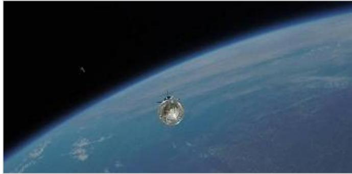
Surprisingly, in less than two minutes after the launch of a 17.7-metre Black Brant IX sounding rocket, a payload separated and began its dive back through Earth's atmosphere. It was the fastest inflation in history of a parachute of this size and created a peak load of almost 70,000 pounds of force.
