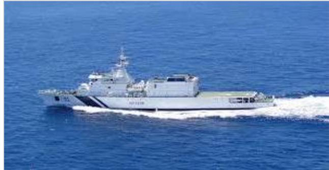
The ship is designed and fully equipped with new technology including Integrated Bridge System (IBS), Automated Power Management System (APMS), Integrated Platform Management System (IPMS), and High Power External Firefighting System (EFFS). It will carry twin engine helicopter (one), and four high speed boats, including two inflatable boats, etc.
