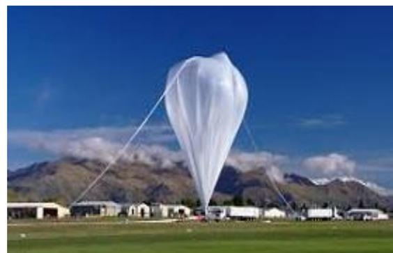
The 532,000 cubic meter balloon is expected to circumnavigate the globe about the southern hemisphere's mid-latitudes once every one to three weeks, depending on wind speeds in the stratosphere and remain airborne for more than 100 days. Long-duration balloon flights provide inexpensive access to the near-space environment for science and technology.
