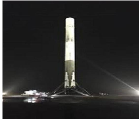
The SpaceX is striving to perfect the technique of landing the booster rockets, making them as reusable as aircraft rather than dumping the expensive equipment into the ocean after each launch.
