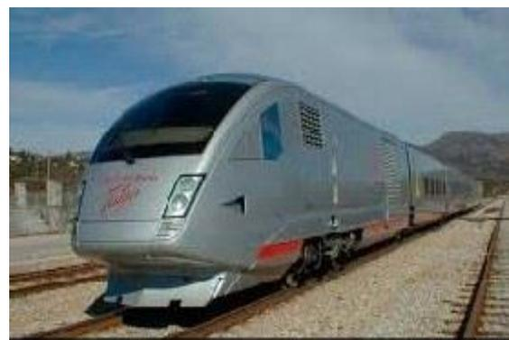
Talgo is a Spanish leading manufacturer of semi-high speed (160-250 kmph) and high-speed (350 kmph) passenger trains. It consumes 30% less energy and can run on curves without decelerating.
