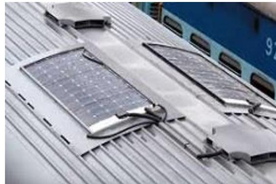
A Noida-based firm Jakson Engineers Limited (JEL), which was awarded a Rs 1.57-crore contract last October by the Indian Railways Organisation for Alternate Fuels for fitting solar panels on 50 DEMU coaches, has completed the work on one rake of Diesel Electric Multiple Unit (DEMU), which has six coaches.
