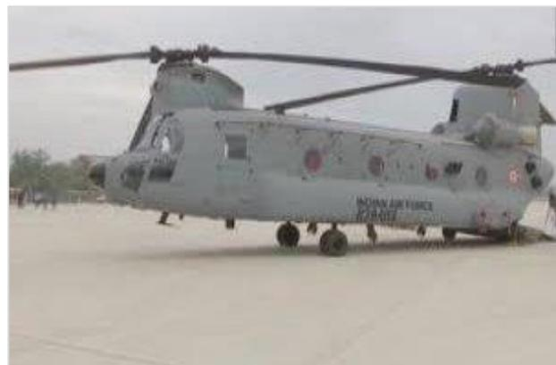
Regarded as one of the most modern heavy lift chopper, the payload capacity of Chinook is about 10 tonne, as it is able to lift artillery, vehicles, road construction and engineer equipment as well as troops and supplies to mountainous sectors. It can also lift M-777 ultra-light howitzers of the Indian armed forces.
