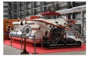
The DSRV system consists of a Submarine Rescue Vessel, a Remote Operations Vehicle,
