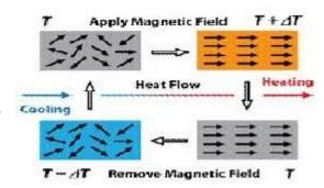
The advantage of magneto-caloric materials which heat up or cool down with the application and removal of the magnetic field, respectively is that as soon as the magnetic field is removed, cooling effect is generated.
