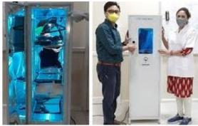
A compact UVC disinfection cabinet consists of four UVC lamps of 30W (on sides) and two lamps of 15~W (top and bottom). The irradiance intensity is measured at various points within the box to assure sufficient radiation to disinfect all the placed articles within 10~minutes.
