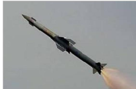
The technology of nozzle less booster has been successfully demonstrated in the mission for the first time in the country. SFDR is a propulsion technology different than that of conventional solid fuelled or liquid fuelled missiles.
