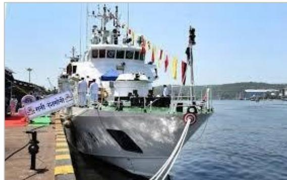
ICGS Rani Rashmoni has been designed and built by the Hindustan Shipyard Limited (HSL) indigenously. It is propelled by three MTU 40000 series diesel engines of 2720 KW capacity each coupled with three Rolls Royce Kamewa jets and can achieve a maximum speeds of 34 knots (63 kmph).
