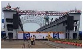
up to 8000 Tons displacement. The dock covers provided with the FDN-2 facilitate repair & refit activities in inclement weather conditions.
