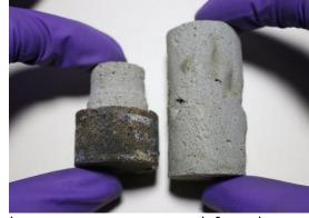
moon surface in future. The process developed now uses urea sourced from human urine, which could be mixed with lunar soil to build structures on the moon.
