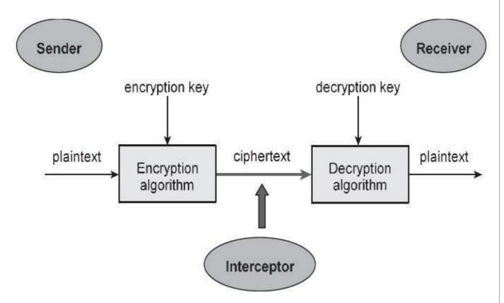
The illustration shows a sender who wants to transfer some sensitive data to a receiver in such a way that any party intercepting or eavesdropping on the communication channel cannot extract the data.
