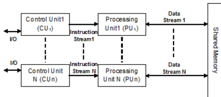
A normal multiprocessor uses the MIMD architecture. These architectures are basically used in a number of application areas such as computer-aided design/computer-aided manufacturing, simulation, modeling, communication switches, etc.
