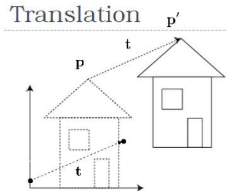
A point can be translated in 3D by adding translation coordinate  $(t_x, t_y, t_z)$  to the original coordinate  $X, Y, Z$  to get the new coordinate  $X', Y', Z'$ .
