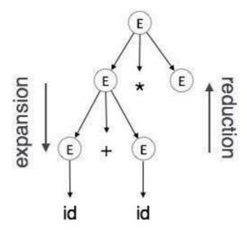
**Reduction**: When a terminal is reduced to its corresponding non-terminal according to grammar rules. Syntax trees are parsed top-down and left to right. Whenever reduction occurs, we apply its corresponding semantic rules *actions*.
