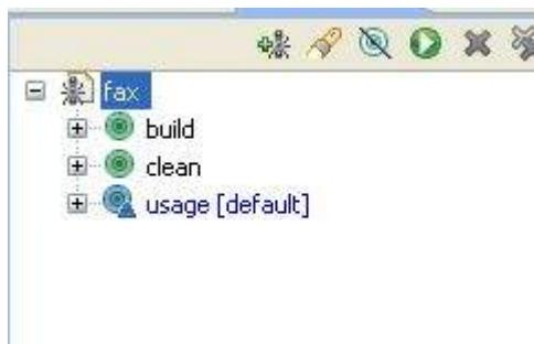
Clicking on the targets, build / clean / usage will run Ant with the target.
