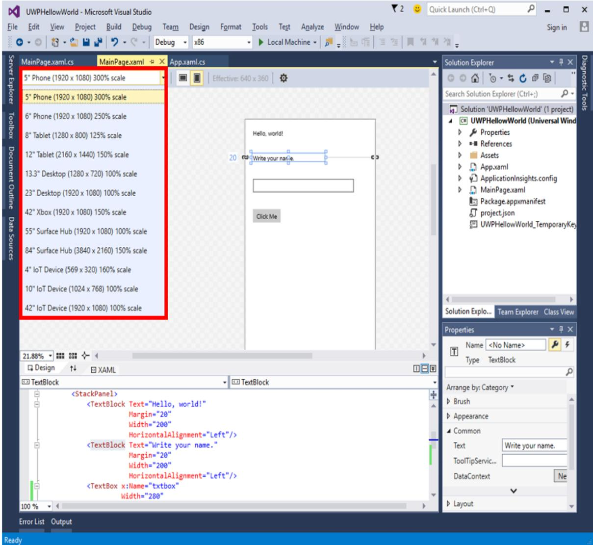
16. You can run and test your app either on a local machine, a simulator or an emulator, or on a remote device. You can select the target device from the following menu as shown below:
