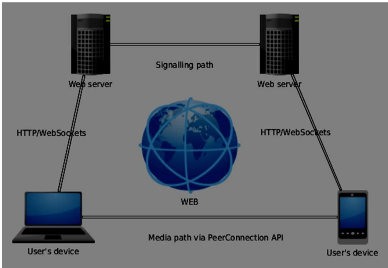
In this model, both devices are running a web application from different servers. The `RTCPeerConnection` object configures streams so they could connect to each other, peer-to-peer. This signaling is done via HTTP or WebSockets.
