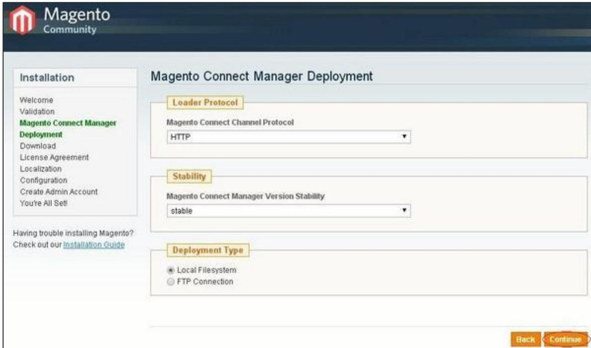
It gives protocol name (HTTP or FTP), stability version such as *stable*, *beta*, *alpha* and deployment type. Select proper options and click on the **Continue** button. It will start the downloading process for Magento.
