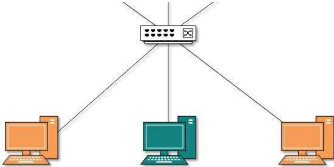
In this diagram, different VLANs are depicted in different color codes. Hosts in one VLAN, even if connected on the same Switch cannot see or speak to other hosts in different VLANs. VLAN is Layer-2 technology which works closely on Ethernet. To route packets between two different VLANs a Layer-3 device such as Router is required.
