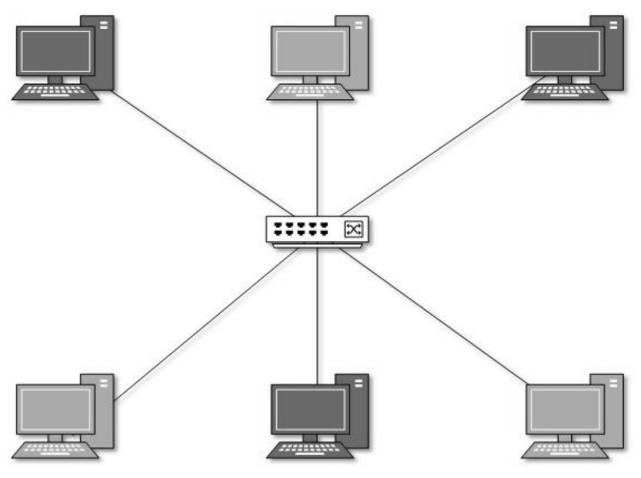
In this diagram, different VLANs are depicted in different color codes. Hosts in one VLAN, even if connected on the same Switch cannot see or speak to other hosts in different VLANs. VLAN is Layer-2 technology which works closely on Ethernet. To route packets between two different VLANs, a Layer-3 device such as Router is required.
