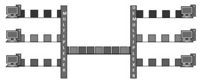
When channel A transmits its frame at one end, the De-multiplexer provides media to channel A on the other end. As soon as the channel A's time slot expires, this side switches to channel B. On the other end, the De-multiplexer works in a synchronized manner and provides media to channel B. Signals from different channels travel the path in interleaved manner.
