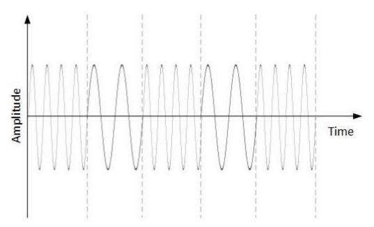
This technique uses two frequencies, f1 and f2. One of them, for example f1, is chosen to represent binary digit 1 and the other one is used to represent binary digit 0. Both amplitude and phase of the carrier wave are kept intact.
