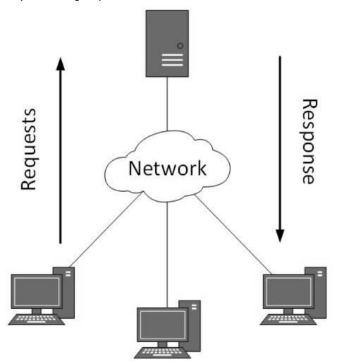
A system can act as Server and Client simultaneously. That is, one process is acting as Server and another is acting as a client. This may also happen that both client and server processes reside on the same machine.
