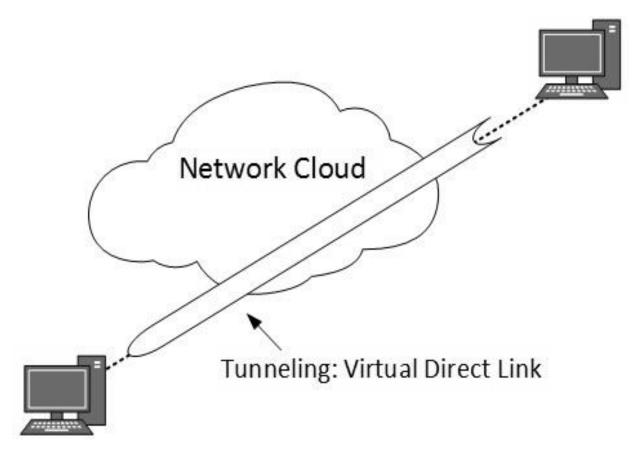
When the data enters from one end of Tunnel, it is tagged. This tagged data is then routed inside the intermediate or transit network to reach the other end of Tunnel. When data exists the Tunnel its tag is removed and delivered to the other part of the network.
