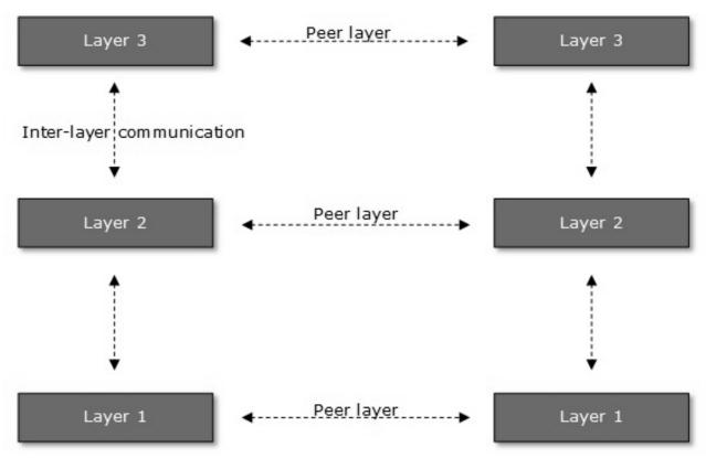
Every layer clubs together all procedures, protocols, and methods which it requires to execute its piece of task. All layers identify their counterparts by means of encapsulation header and tail.
