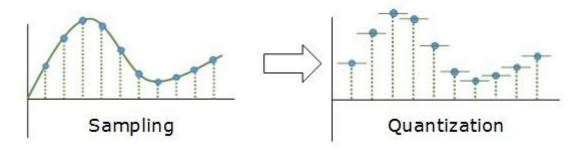
Sampling yields discrete form of continuous analog signal. Every discrete pattern shows the amplitude of the analog signal at that instance. The quantization is done
