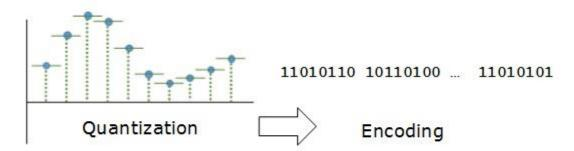
In encoding, each approximated value is then converted into binary format.
