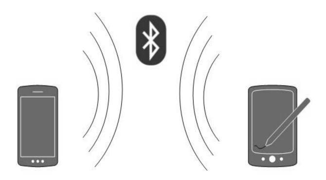
For example, Piconet is Bluetooth-enabled Personal Area Network which may contain up to 8 devices connected together in a master-slave fashion.
