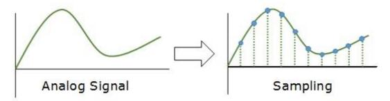
The analog signal is sampled every T interval. Most important factor in sampling is the rate at which analog signal is sampled. According to Nyquist Theorem, the sampling rate must be at least two times of the highest frequency of the signal.
