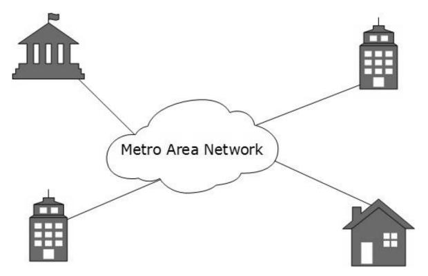
Backbone of MAN is high-capacity and high-speed fiber optics. MAN works in between Local Area Network and Wide Area Network. MAN provides uplink for LANs to WANs or internet.
