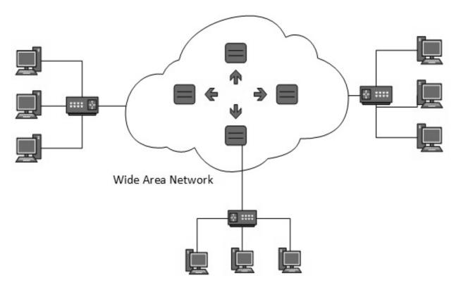
WAN may use advanced technologies such as Asynchronous Transfer Mode (ATM), Frame Relay, and Synchronous Optical Network (SONET). WAN may be managed by multiple administration.
