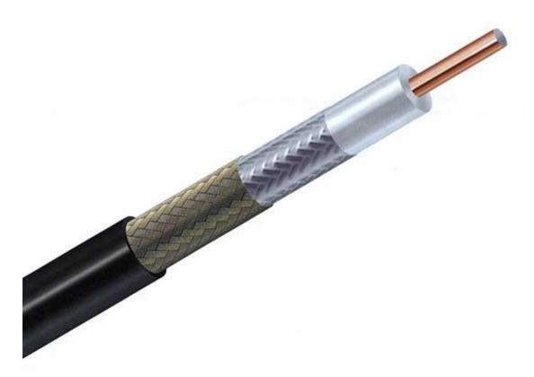
Because of its structure, the coax cable is capable of carrying high frequency signals than that of twisted pair cable. The wrapped structure provides it a good shield against noise and cross talk. Coaxial cables provide high bandwidth rates of up to 450 mbps.
