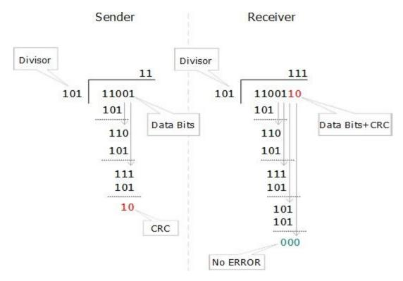
At the other end, the receiver performs division operation on codewords using the same CRC divisor. If the remainder contains all zeros the data bits are accepted, otherwise it is considered as there is some data corruption occurred in transit.
