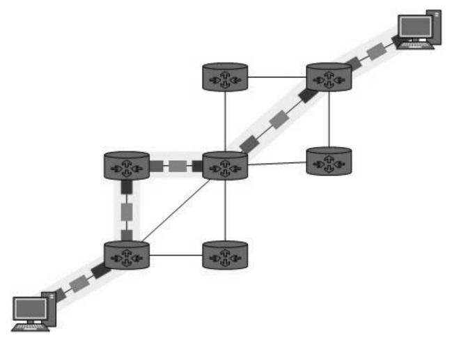
Circuit switching was designed for voice applications. Telephone is the best suitable example of circuit switching. Before a user can make a call, a virtual path between caller and callee is established over the network.
