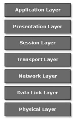
**Application Layer:** This layer is responsible for providing interface to the application user. This layer encompasses protocols which directly interact with the user.
