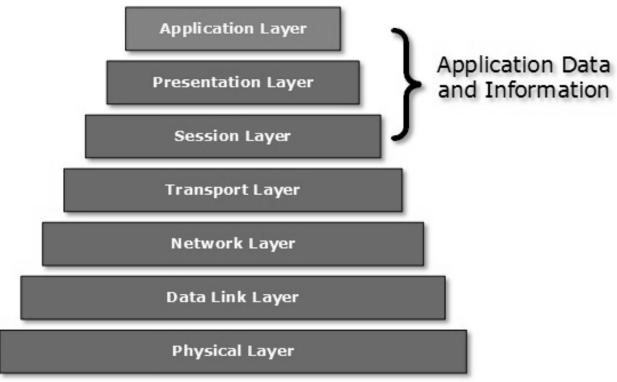
There is an ambiguity in understanding Application Layer and its protocol. Not every user application can be put into Application Layer except those applications which interact with the communication system. For example, designing software or texteditor cannot be considered as application layer programs.
