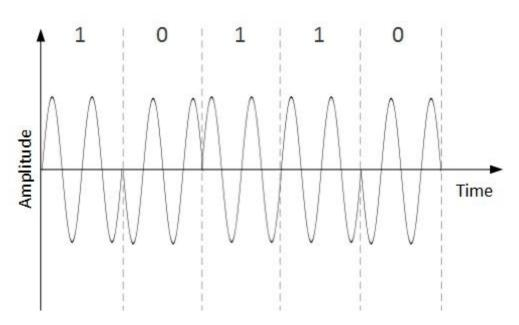
When a new binary symbol is encountered, the phase of the signal is altered. Amplitude and frequency of the original carrier signal is kept intact.
