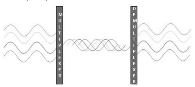
Further, on each wavelength time division multiplexing can be incorporated to accommodate more data signals.
