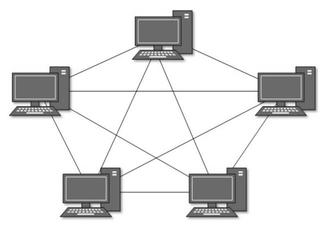
Hosts in Mesh topology also work as relay for other hosts which do not have direct point-to-point links. Mesh technology comes into two types:
