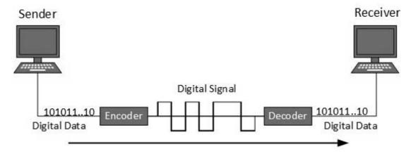
Digital signal is denoted by discreet signal, which represents digital data. There are three types of line coding schemes available:
