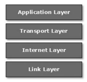
**Application Layer:** This layer defines the protocol which enables user to interact with the network. For example, FTP, HTTP etc.
