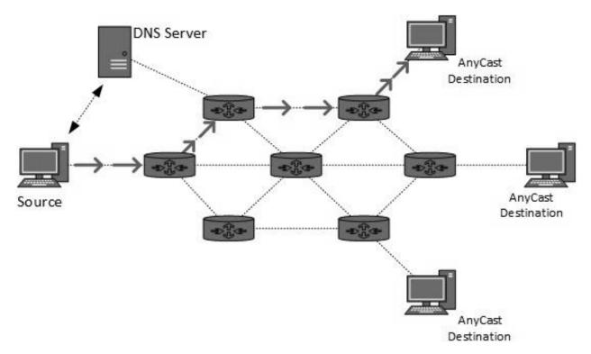
Anycast routing is done with help of DNS server. Whenever an Anycast packet is received it is enquired with DNS to where to send it. DNS provides the IP address which is the nearest IP configured on it.
