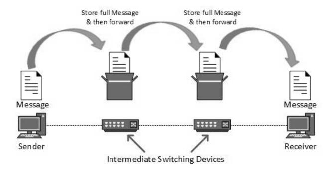
This technique was considered substitute to circuit switching. As in circuit switching the whole path is blocked for two entities only. Message switching is replaced by packet switching. Message switching has the following drawbacks:
